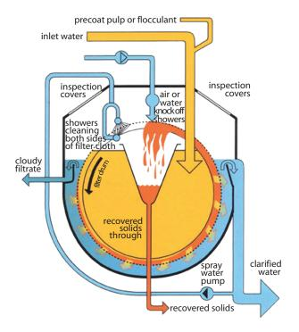
ALGAS Microfilters reclaims over 95% of all suspended solids.
