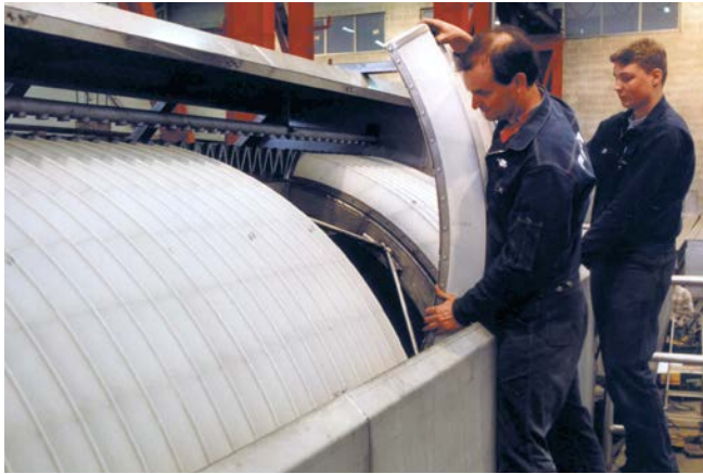
Easy replacement of segments for cloth changing.
